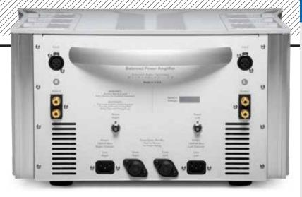
**ABOVE:** Truly dual mono, with two IEC mains inlets feeding two independent PSUs (and with two replaceable fuses). Balanced inputs on XLRs only, with speaker outputs on 4mm binding posts. Buttons allow manual re-setting of the electronic protection
