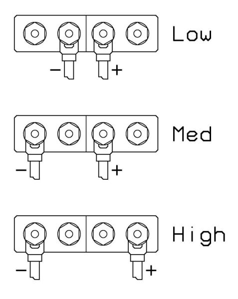
Figure 1 Output Connections
