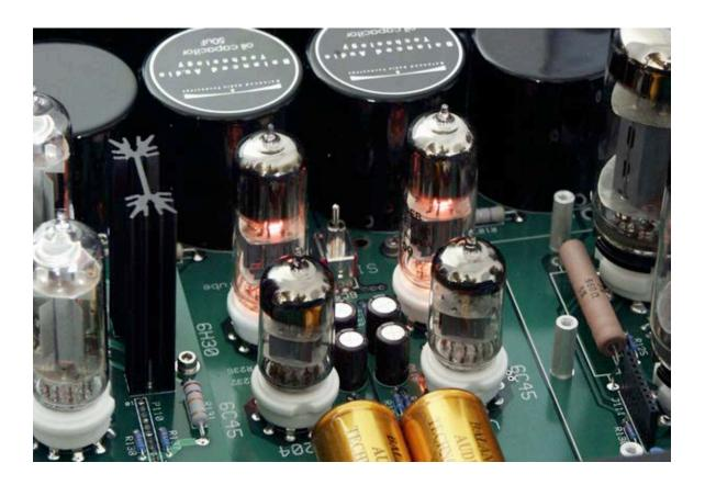
They incorporate two types of vacuum tubes, user selectable for the desired sound: 6C45 and 6H30.
