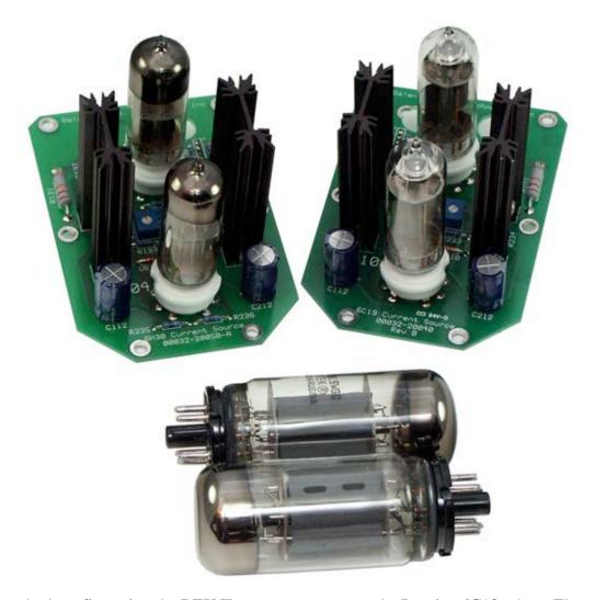
In its standard configuration the REX II current sources use the Russian 6C19 tubes. That tube is basically a miniature version of the famous 6C33 tube, and provides, in our view, the best combination of sonic characteristics and electrical performance.
