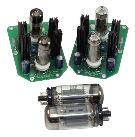
In its standard configuration the VK-32SE current sources use the Russian 6C19 tubes. That tube is basically a miniature version of the famous 6C33 tube, and provides, in our view, the best combination of sonic characteristics and electrical performance.
