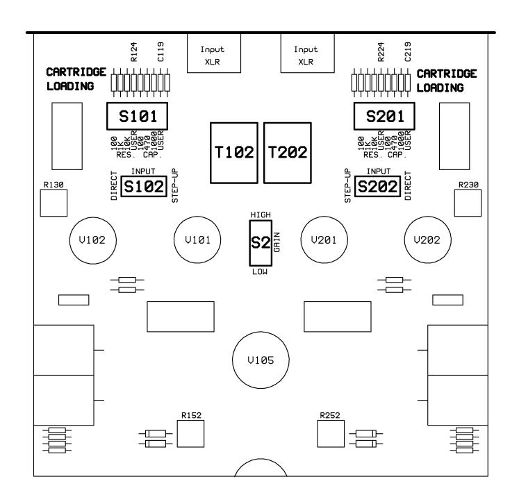
Figure 1: UK-P10 Internal Controls
